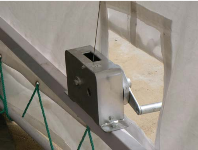
Winch Assembly Mounted To Lower End panel Beam
