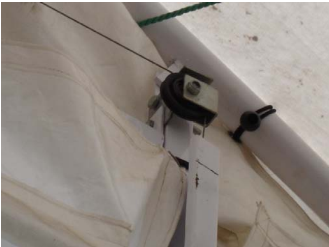
Single Door Pulley Farthest From Winch Assembly
