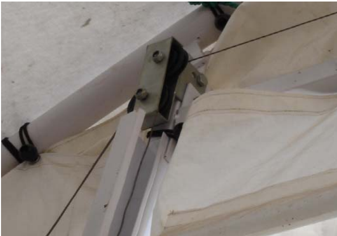
Double Pulley Nearest Winch Assembly
