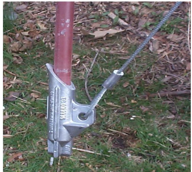
Drive Rod inserts into Anchor Head
