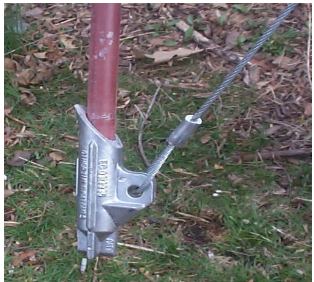
Drive Rod inserts into Anchor Head
